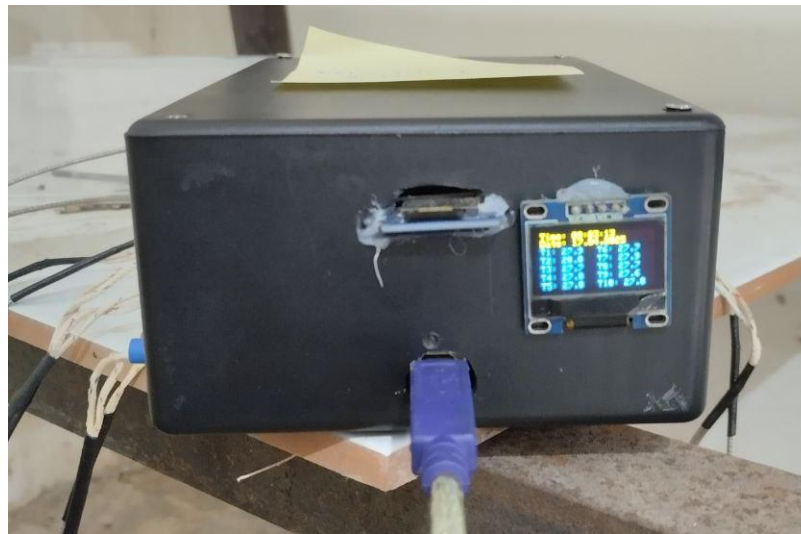
Gambar 2. Sistem monitoring suhu 10 channels
