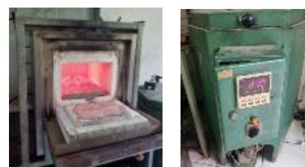
Gambar 3. a) Hardening, b) Tempering
