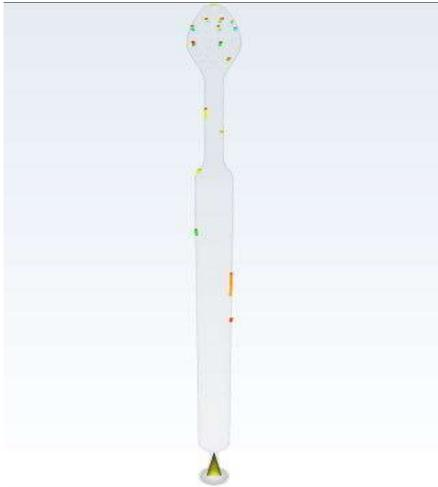
Gambar 5. Cacat weld line lokasi gate 2.
