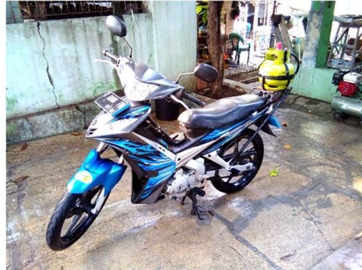
Gambar 1. Sepeda motor Yamaha Jupiter MX bi-fuel.
