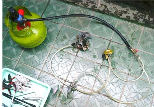
Gambar 8. Skema konverter kit bi-fuel.
